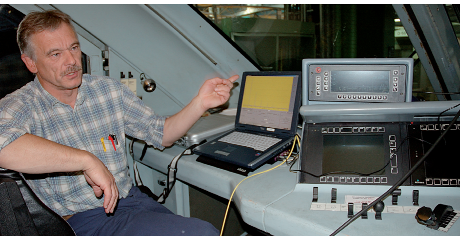
Rail vehicle electrician Hans-Günter Thomas with the C-OTDR in the power car of an ICE 1. The C-OTDR's hardware lies under the laptop console. The software runs on his colleague's laptop. That way, he can save reference curves and observe gradual changes when the train is next serviced at the plant.
